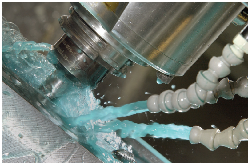
Figure 1 | Boundary lubricity additives are widely used in metalworking fluid applications. Their selection is particularly critical in high-temperature and pressure applications. [Courtesy of The Lubrizol Corp.]
